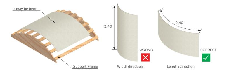
The 8 mm thick Cementex board gives the possibility to produce curved surfaces with a minimum radius of curvature of 8 m on the long direction of the slab. To obtain such a curve, the board should be well moistened, with a constant load applied on a support frame.
