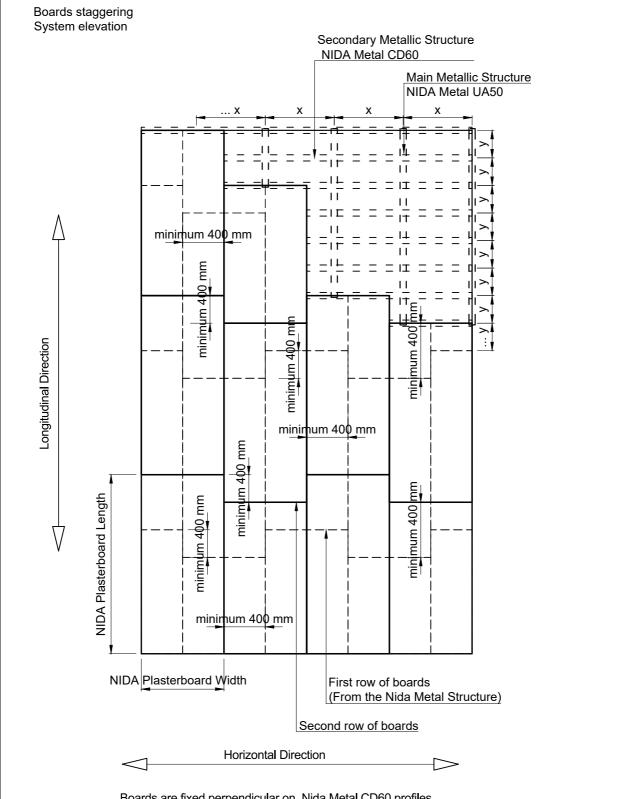
Boards are fixed perpendicular on Nida Metal CD60 profiles. Boards staggering on longitudinal direction is minimum 400 mm.
