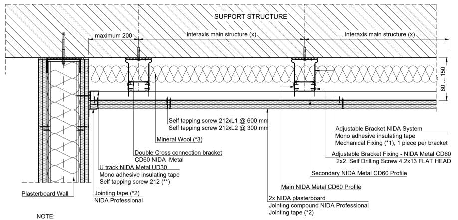
(\*\*) The self tapping screw shall be fixed on the metal structure of the Plasterboard Wall, the length of the screw will be according to the thikness of the fixing package (Wall boards thikness of layers)
