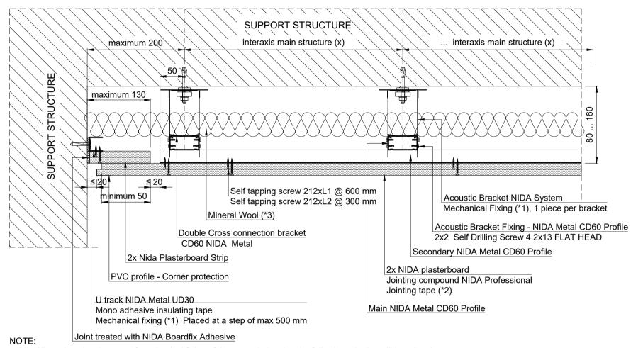
(\*1) When choosing the type of mechanical fixing of the acoustic bracket the following criterias will be taken into account:
