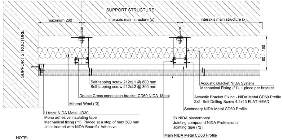
(\*1) When choosing the type of mechanical fixing of the acoustic bracket the following criterias will be taken into account:
