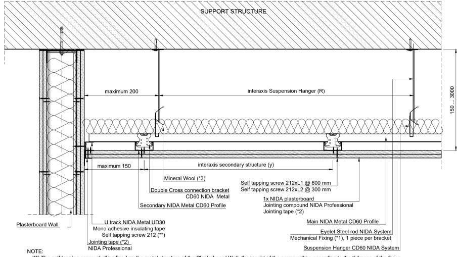
(\*\*) The self tapping screw shall be fixed on the metal structure of the Plasterboard Wall, the lenght of the screw will be according to the thikness of the fixing package (Wall boards thikness of layers)
