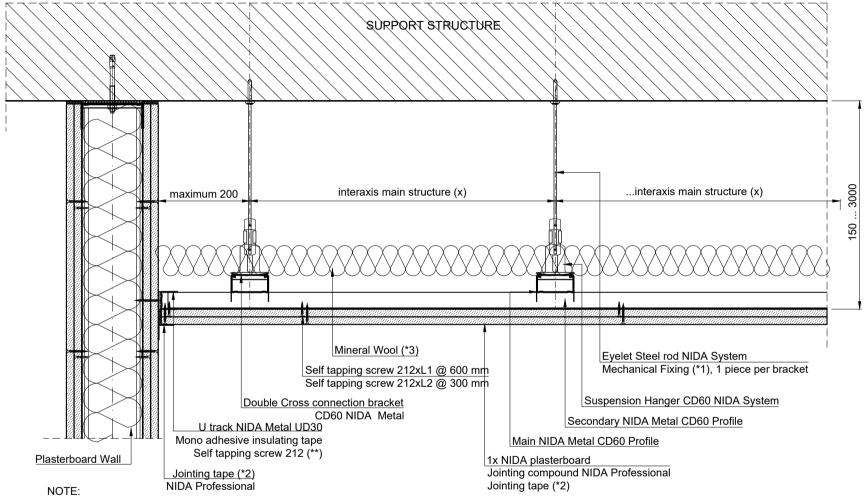
(\*\*) The self tapping screw shall be fixed on the metal structure of the Plasterboard Wall, the length of the screw will be according to the thikness of the fixing package (Wall boards thikness of layers)
