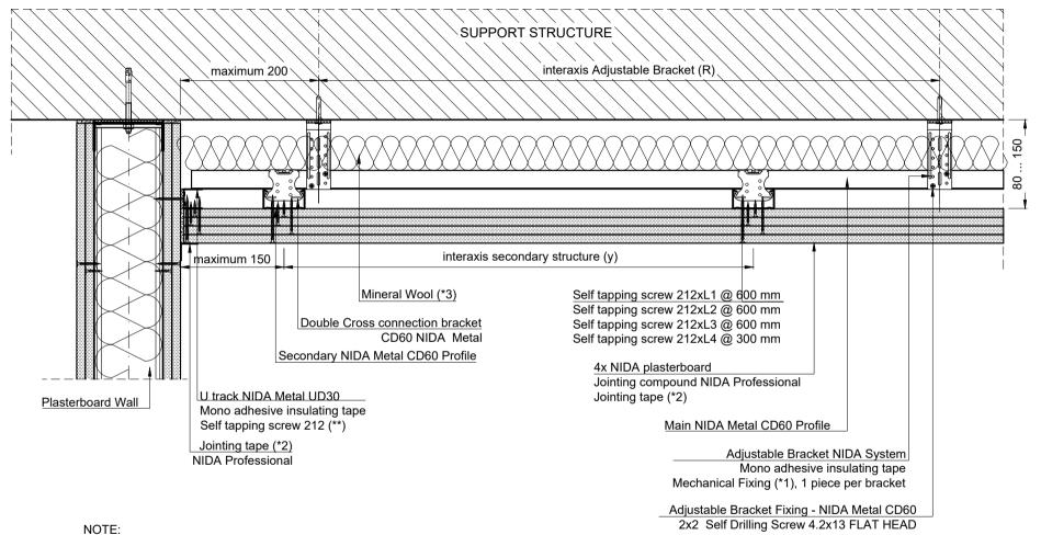
(\*\*) The self tapping screw shall be fixed on the metal structure of the Plasterboard Wall, the length of the screw will be according to the thikness of the fixing package (Wall boards thikness of layers)
