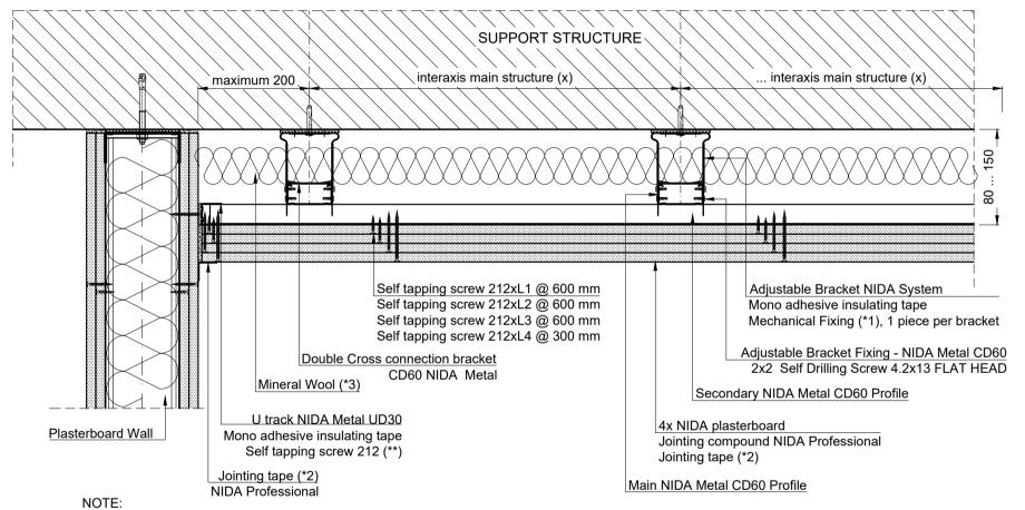
(\*\*) The self tapping screw shall be fixed on the metal structure of the Plasterboard Wall, the length of the screw will be according to the thikness of the fixing package (Wall boards thikness of layers)
