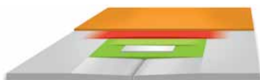
Q2 + 1 layer of plaster over the entire surface of the board
